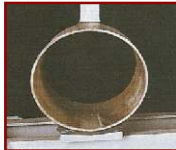
Crush resistance of a PRY pipe
