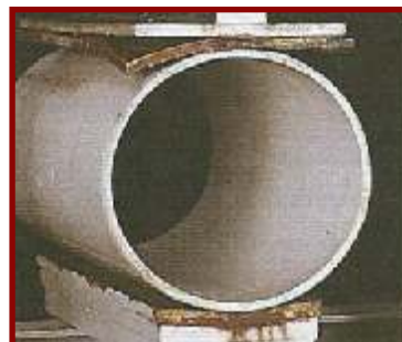
Crush resistance of a PVC pipe
